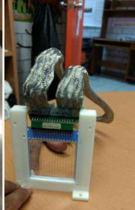
2 (of 4) Double-sided silicon strip detectors (DSSSD) 20 micron. 16x16 strips, 5x5 cm active area.
