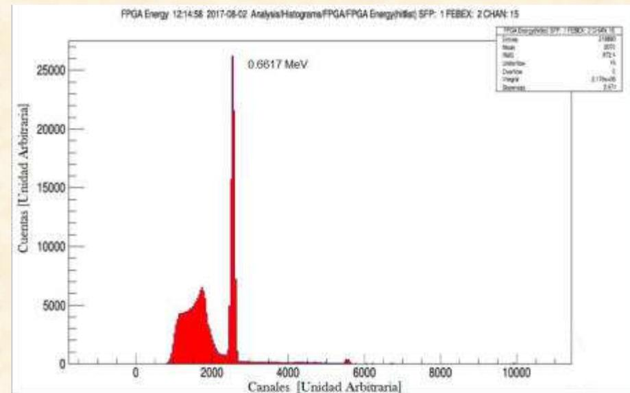
$^{137}\text{Cs}$  in a Germanium detector.
