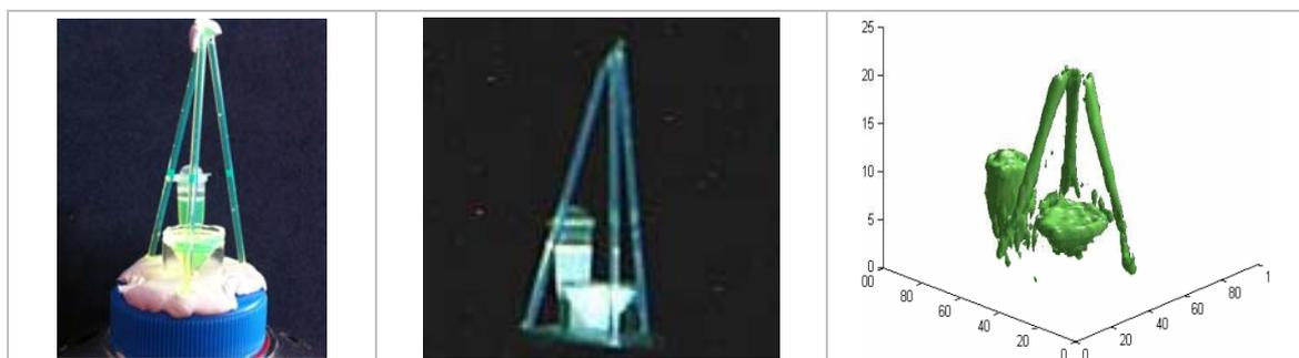
**Figure 3:** Left: A picture of the optical phantom with fluorescent liquid (Cyalume) – Middle: A planar image obtained by the CCD-Camera – Right: The 3D reconstructed image of the optical phantom.
