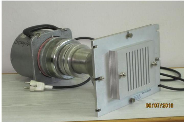
Observation and Measurement can be done with a six stage HV Cascade Impactor. A device that sucks air in order to collect and divide radioactive aerosols by size. This classification occurs due to the different cuts of the metal plates and the way they affect the air streamline passing through. The filters we use are made of fiberglass material.
