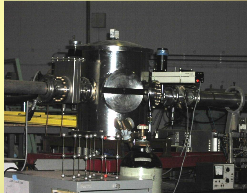
The H.V.E. 5.5 MV Tandem vdG accelerator of the NCSR Demokritos (Athens) and the utilized Charles Evans & Assoc. scattering chamber
