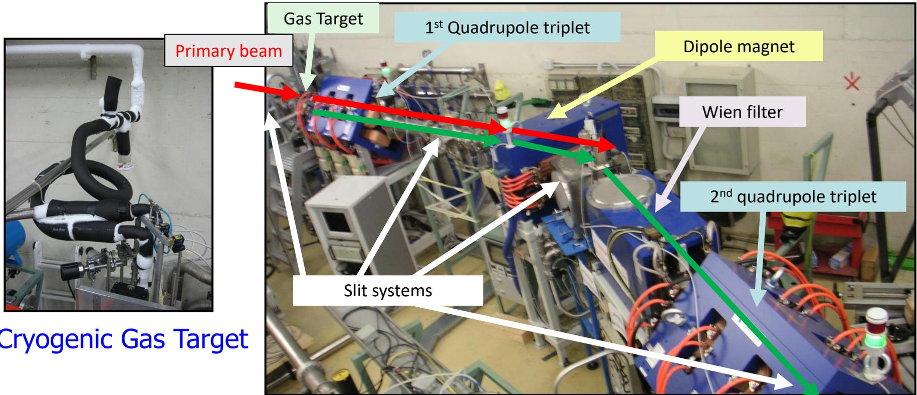
Cryogenic Gas Target
