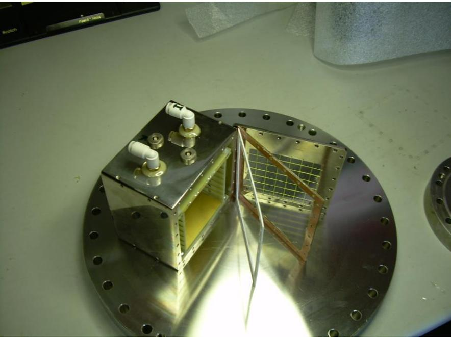
Easy handling, thickness uniformity, possibility to tune the effective thickness, large detection surface, no radiation damage problems, low thresholds
