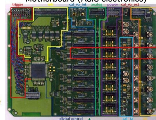
Innovative readout electronics by means of an 32-channel ASIC chip manufactured by IDEAS-GM (Norway) dedicated to the treatment of the linear and the logical part of the electronic signals coming from the detector strips.
