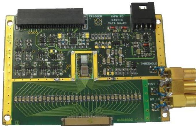
Motherboard (ASIC electronics)
