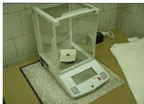
**Figure 3.6.** The balance where the pills of mosses were weighted. Only 0.3 g of moss material is required for the ENAA.
