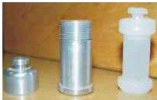
**Figure 3.25.** Transport capsules for irradiation.
