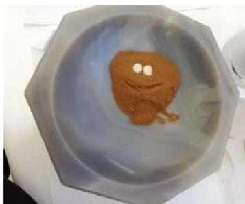
**Figure 3.9.** The sieved soil with the wax, before the homogenization and the creation of the pressed pellet.
