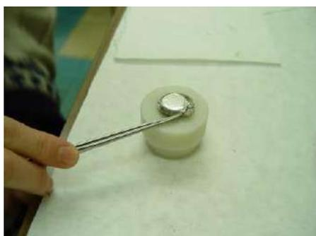
**Figure 3.7.** Preparing the aluminum foil cups for long-term irradiation.
