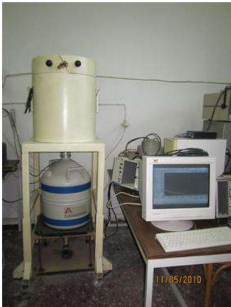
**Figure 3.14.** The HPGe 20% relative efficiency detector.
