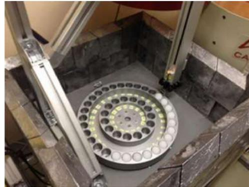
**Figure 3.28.** The disk with the slots for containers.
