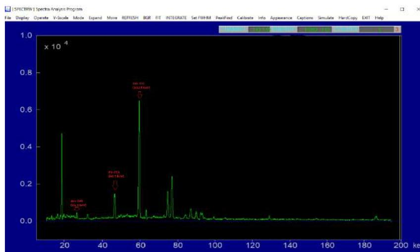
**Figure 3.19.** Gamma spectrum of IAEA-CU-2006 reference material. The peaks of 26.34 keV ( $^{241}\text{Am}$ ), 59.54 keV ( $^{241}\text{Am}$ ) and 46.5 keV ( $^{210}\text{Pb}$ ) are presented.
