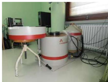
**Figure 3.13.** The HPGe detector with 100% relative efficiency.
