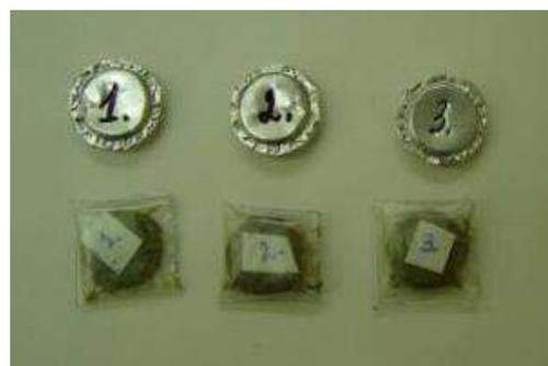
**Figure 3.8.** The plastic bags where the pills were put for short-term irradiation and the aluminum foil cups for long-term irradiation.
