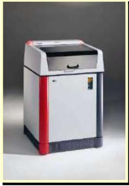
**Figure 3.33.** The X-ray Spectrometry S4-Pioneer (Bruker-AMS, Deutschland) was used for the determination of trace elements content in 95 soil samples.
