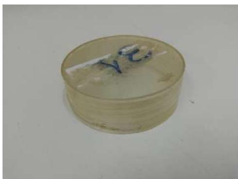
**Figure 3.17.** The *small* box that was used for gamma measurements.
