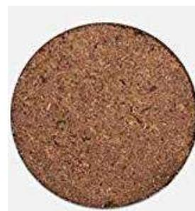
**Figure 3.11** The pressed pellet that was used for the XRF measurements.
