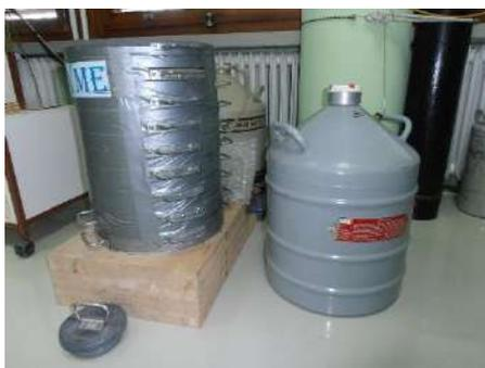
**Figure 3.12.** The low-background extended range HPGe detector equipped with a Be window.
