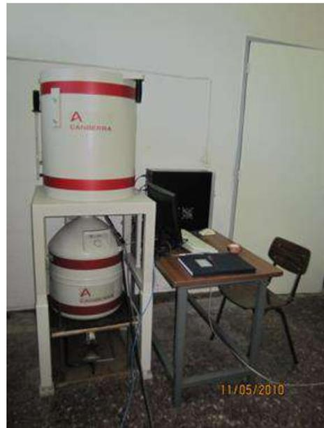
**Figure 3.15.** The HPGe 42% relative efficiency detector.
