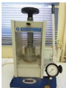
**Figure 3.10.** The manual pneumatic press system that was used for the creation of the pellets. Pressure of 15 tons was performed for each soil sample.
