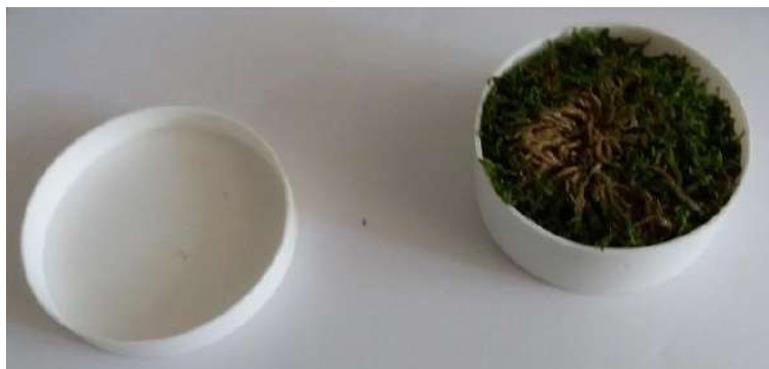
**Figure 3.4.** The moss sample placed in plastic cylindrical container for measurement of gamma spectra.
